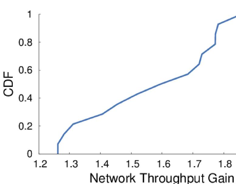
MiRa's MU-MIMO increases the network throughput by an average of 1.6x
